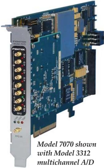
Model 7070 shown with Model 3312 multichannel A/D & D/A FMC module
